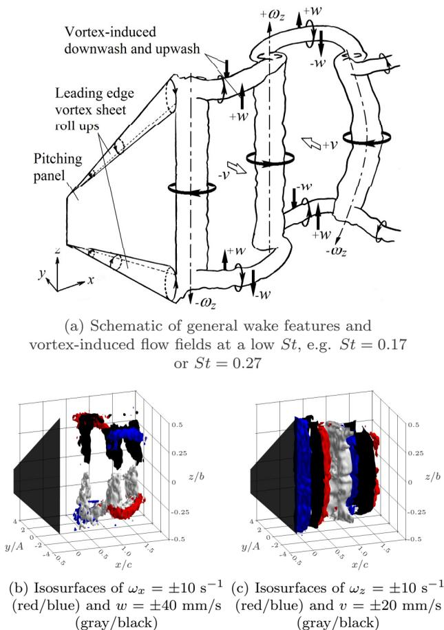
FIG. 8. Schematic of general wake features and vortex-induced flow fields, and isosurfaces obtained from PIV data. Isosurfaces of  $\omega_x$ ,  $\omega_z$ ,  $v$ , and  $w$  are shown for  $St = 0.27$  at  $t/T = 0$ .
