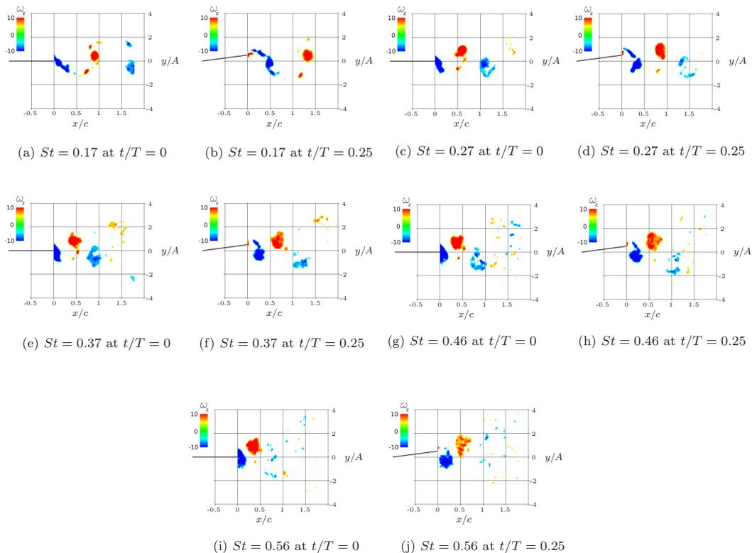
FIG. 7. Top views of  $\omega_z$  in the plane of the midspan at  $t/T = 0$  (left column) and  $t/T = 0.25$  (right column) for all five  $St$ . The plots have been thresholded in order to only display regions of the wake where  $|\omega_z| \geq 5 \text{ s}^{-1}$ .
