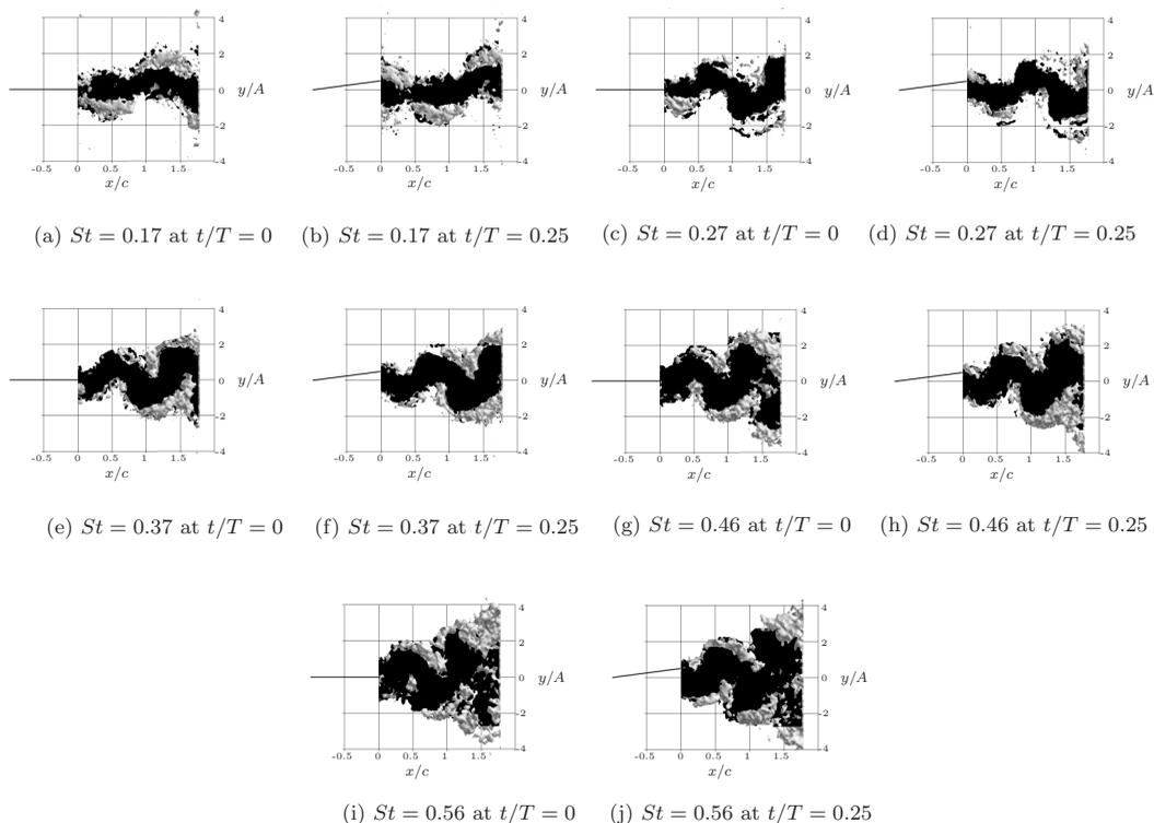
FIG. 10. Top views of  $w$  isosurfaces at  $t/T = 0$  (left column) and  $t/T = 0.25$  (right column) for all five  $St$ . Gray isosurfaces are presented at  $w = 25$  mm/s and black isosurfaces are presented at  $w = -25$  mm/s.
