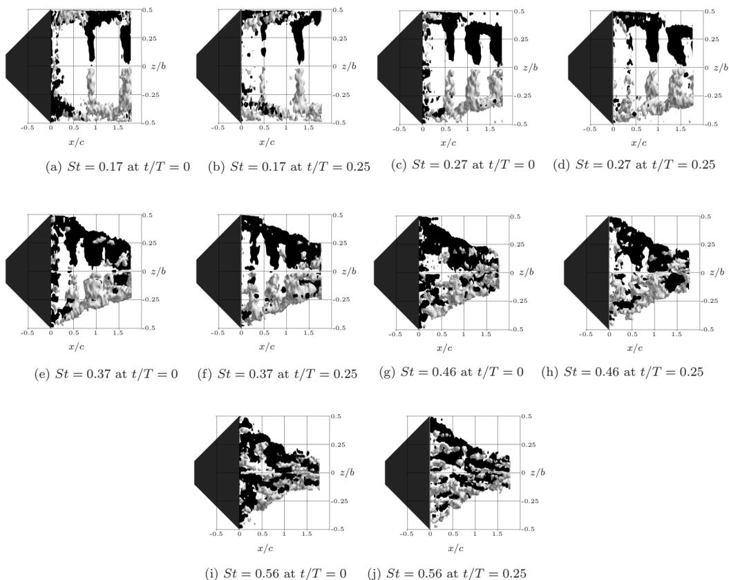
FIG. 9. Side views of  $w$  isosurfaces at  $t/T = 0$  (left column) and  $t/T = 0.25$  (right column) for all five  $St$ . Gray isosurfaces are presented at  $w = 25$  mm/s and black isosurfaces are presented at  $w = -25$  mm/s.
