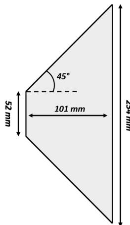
FIG. 2. Geometric details of the trapezoidal pitching panel.
