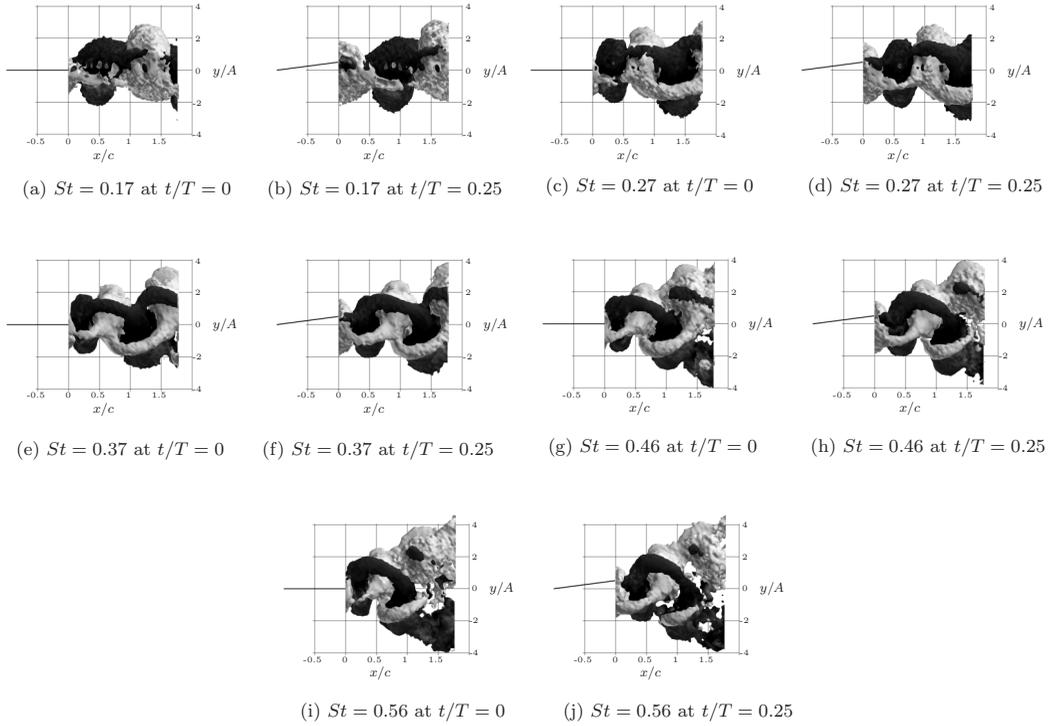
FIG. 13. Top views of  $v$  isosurfaces at  $t/T = 0$  (left column) and  $t/T = 0.25$  (right column) for all five  $St$ . Gray isosurfaces are presented at  $v = 20$  mm/s and black isosurfaces are presented at  $v = -20$  mm/s.
