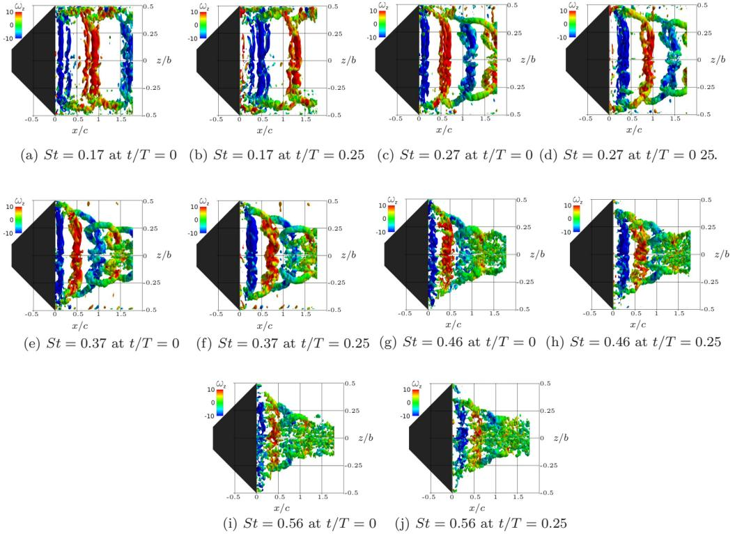
FIG. 4. Side views of  $Q$  isosurfaces at a level of 1%  $Q_{\max}$  at  $t/T = 0$  (left column) and  $t/T = 0.25$  (right column) for all five  $St$ .  $Q$  isosurfaces are colored by the local value of  $\omega_z$ .
