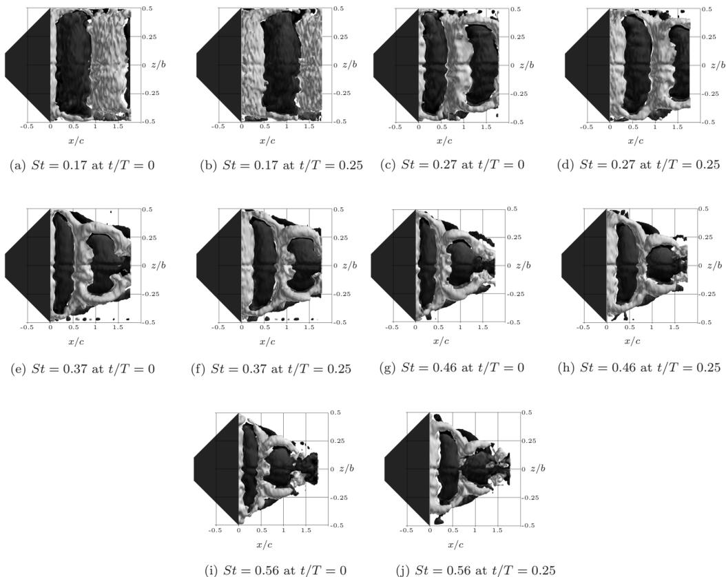
FIG. 12. Side views of  $v$  isosurfaces at  $t/T = 0$  (left column) and  $t/T = 0.25$  (right column) for all five  $St$ . Gray isosurfaces are presented at  $v = 20$  mm/s and black isosurfaces are presented at  $v = -20$  mm/s.
