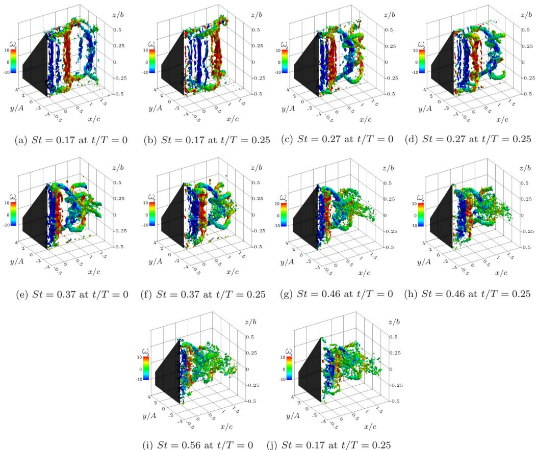
FIG. 3. Isometric views of  $Q$  isosurfaces at a value of 1%  $Q_{\max}$  at  $t/T = 0$  (left column) and  $t/T = 0.25$  (right column) for all five  $St$ .  $Q$  isosurfaces are colored by the local value of  $\omega_z$ .
