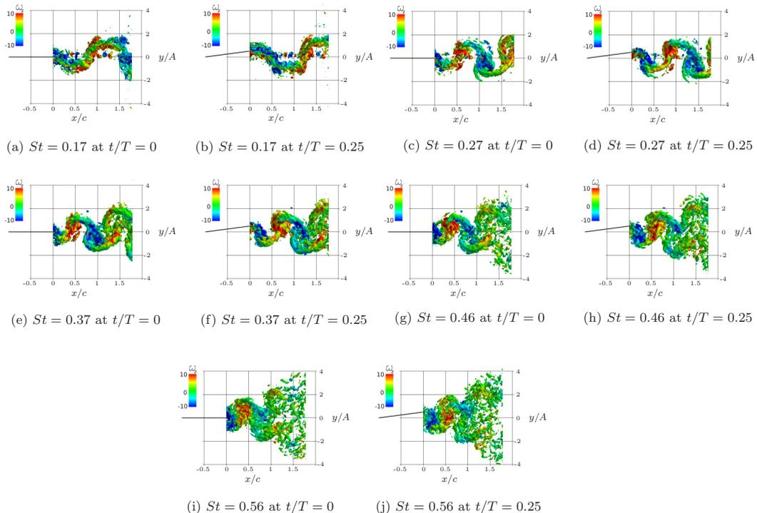
FIG. 6. Top views of  $Q$  isosurfaces at a level of 1%  $Q_{\max}$  at  $t/T = 0$  (left column) and  $t/T = 0.25$  (right column) for all five  $St$ .  $Q$  isosurfaces are colored by the local value of  $\omega_z$ .
