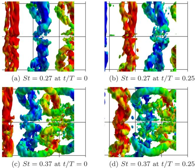
FIG. 5. Zoom-in of side views of  $Q$  isosurfaces at a level of 1%  $Q_{\max}$  at  $t/T = 0$  (left column) and  $t/T = 0.25$  (right column) for  $St = 0.27$  and  $St = 0.37$ . Isosurfaces of  $Q$  are colored by the local value of  $\omega_z$  in the same manner as Fig. 4.
