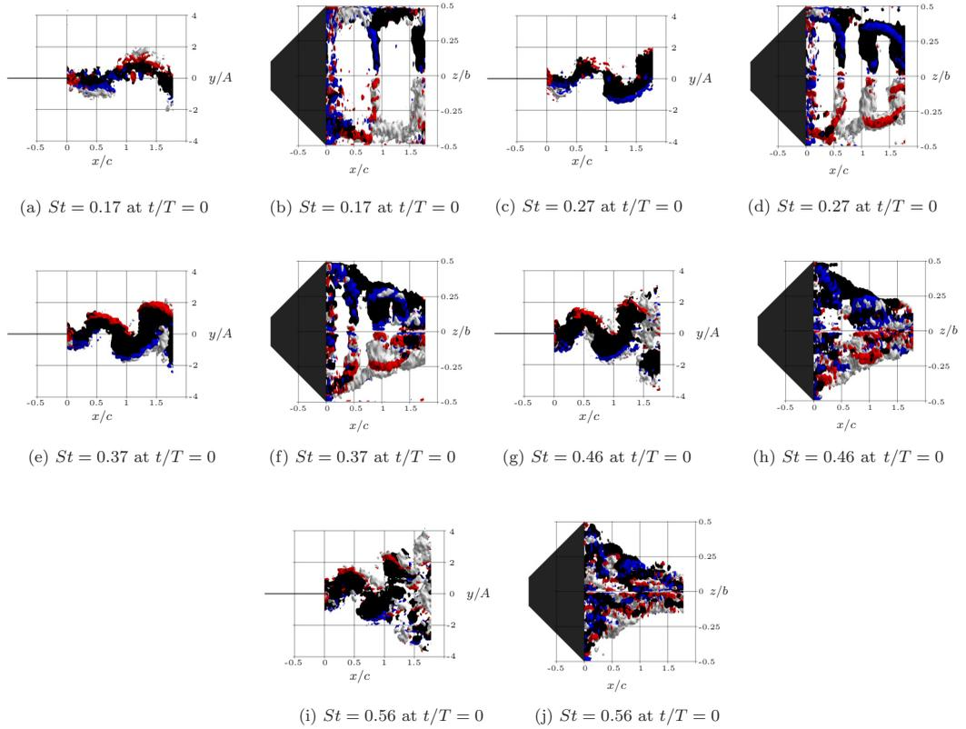
FIG. 11. Top views (left column) and side views (right column) of isosurfaces of  $\omega_x$  and  $w$  at  $t/T = 0$  (left column) for all five  $St$ . Red and blue isosurfaces of  $\omega_x$  are presented at  $\omega_x = 10 \text{ s}^{-1}$  and  $\omega_x = -10 \text{ s}^{-1}$ , respectively. Gray and black isosurfaces of  $w$  are presented at  $w = 40 \text{ mm/s}$  and  $w = -40 \text{ mm/s}$ , respectively.
